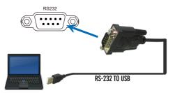
Then, open a Serial Command tool on PC to send ASCII commands to control the Matrix. The ASCII command list of the product is as below.
