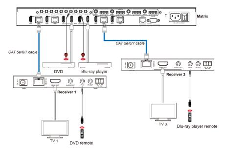
Figure 2: IR connection diagram (HDBaseT Receiver end)
