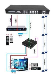
The matrix is not only a switcher and extender of multiple HDMI signals to multiple HDMI receivers located remotely, it also passes IR control signals through the IR call-back system to the matrix and HDMI sources for full, independent control of all connected inputs from output locations.
