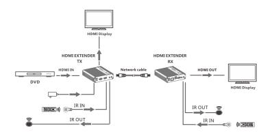
Note: To ensure the quality of signal transmission, please use network cable within 50 meters when cascaded.
