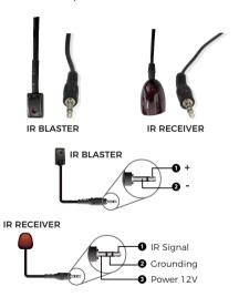
**Note:** When the angle between the IR receiver and the remote control is  $\pm$  45  $^{\circ}$ , the transmission distance is 0-5 meters; when the angle between the IR receiver and the remote control is  $\pm$  90  $^{\circ}$ , the transmission distance is 0-8 meters.
