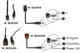
**Note:** When the angle between the IR receiver and the remote control is  $\pm$  45<sup>°</sup>, the transmission distance is 0-5 meters; when the angle between the IR receiver and the remote control is  $\pm$  90<sup>°</sup>, the transmission distance is 0-8 meters.
