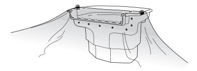
Remove the spring clips and pull the liner away from the face of the enclosure. Make sure that the front of the FilterFalls and the back side of the liner are clean and free of debris. Apply a consistent bead of Atlantic fish-safe RTV silicone to the face of the FilterFalls along the center line of the threaded inserts.
