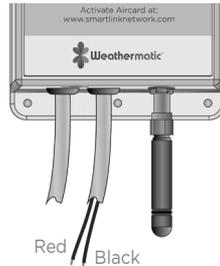
**Note:** The wire connection between the Aircard and the SLFSI Flow Sensor should be made inside the housing of the SmartLine controller, or an enclosure. Only use the provided 3M® Scotchlok™ Connectors. Insert the unstripped wires into the holes of the connector. Use a pair of pliers to make the connection by driving the cap down flush with the top edge of the connector body. Verify wires are secure.
