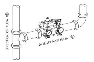
TYPICAL INSTALLATION (MODEL ZW209FP with gauge 2005-25UL)
