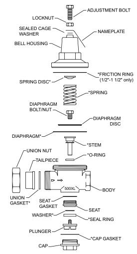
\* INDICATES PARTS SUPPLIED IN REPAIR KITS (spring disc not included in sizes 1 1/2" - 3")
