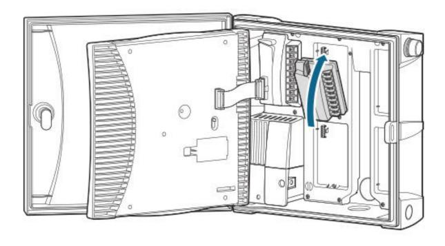
Tip the two tabs on one end of the module into the mating holes in one end of the slot, and tip the module firmly into place.
