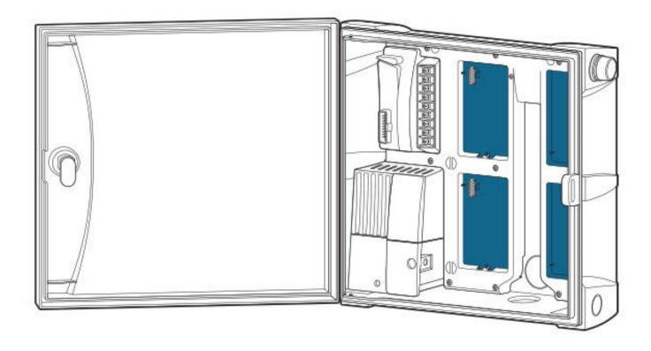
Open the controller inner panel, and choose the next available open slot in the controller. Slots are numbered, down the first column and up the second.
