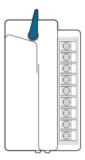
Flip the blue locking lever into the vertical unlocked position.
