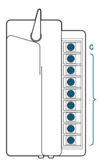
Connect field and common wiring as needed and test.
