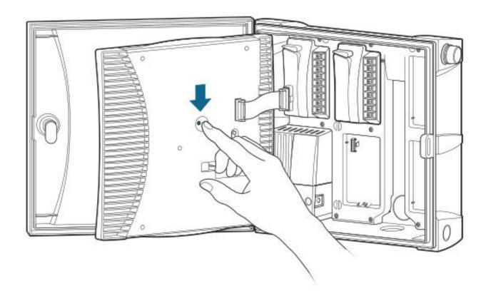
Press the Reset button on the back of the controller control panel. This is required for the controller to recognize the new module.
