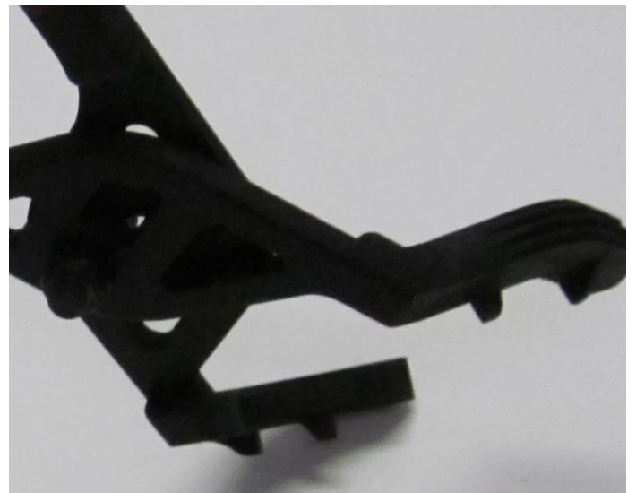
Bottom teeth engage cap fins on rotor and spray heads
