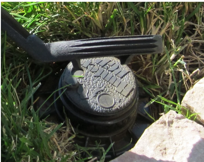
Bottom teeth engage cap fins on rotor and spray heads
