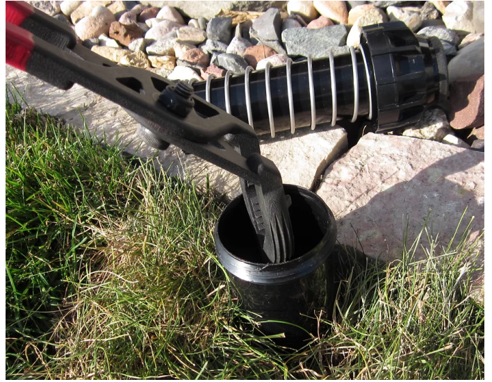
Extract sprinkler bodies and fitting with easy-out teeth
