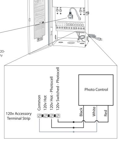
Photo Controls for Vista Transformers
