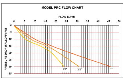
Note: Flow curves are based on static conditions of 100psi inlet pressure and 50 psi outlet pressure. Pressure differential is the difference between the supply pressure and adjusted outlet pressure measured in the static (closed) condition.
