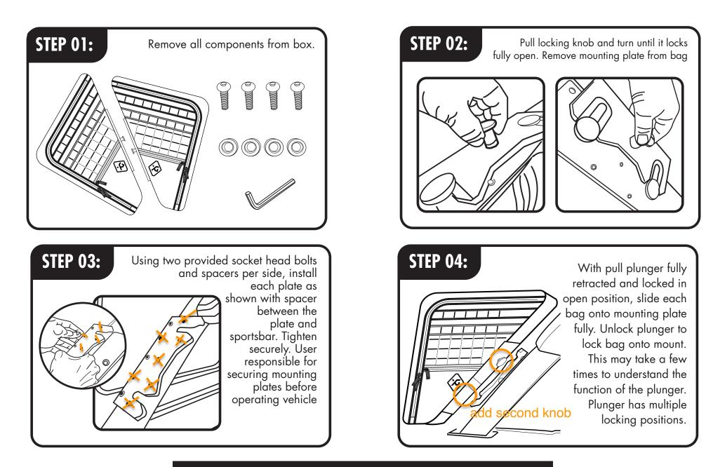
Note: Be sure plunger is fully retracted into open position for installation and removal as damage may occur to coated surfaces.
