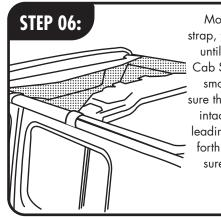
Moving from strap to strap, tighten as needed until Magne-Lok Mesh Cab Shade is tight and smooth while making sure the locator pins are intact. Flip Magne-Lok leading edge back and forth a few times to be sure pins are aligned and operational
