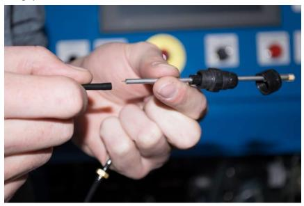
Installing the filter tip assembly on the LACO Sniffer probe
