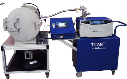
Automated helium hard vacuum leak testing system using a TitanTest™ leak detector, a LACO vacuum test chamber, and an Atlas™ leak test process controller with data logging.
