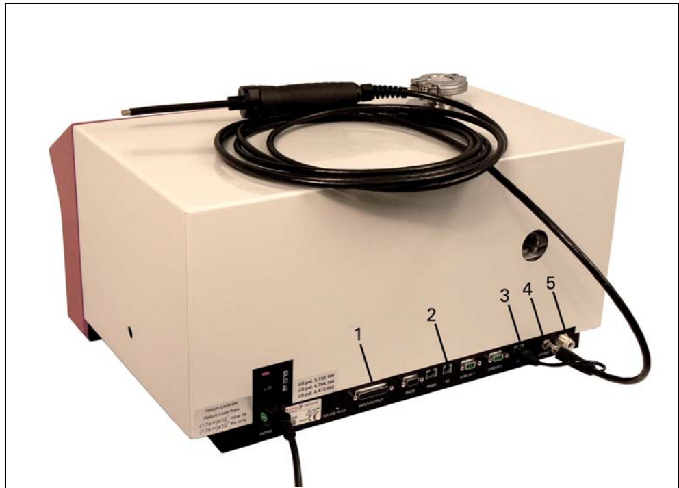
Fig. 5-2 Connections for sniffing probe
