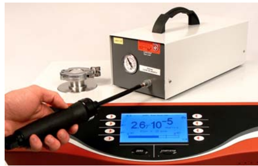
Fig. 6-81 Sniffing external test leak
