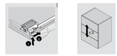
\*NOTE: Runners have a 3mm range of motion in a vertical direction.
