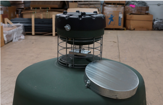
Step 11: Place powerhead on top of cage.
