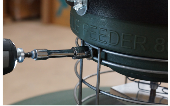
Step 12: Bolt powerhead down.
