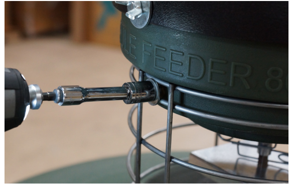
Step 14: Bolt powerhead down. (3) SM Washer (3) Bolt
