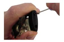
Place recoil pad insert at end of stock. Screw on recoil pad (I) using the 2 longest screws
