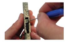
Place short screw into barrel (A) and stock (D) where holes align nearest to top.
