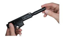
Thread suppressor (D) over muzzle by rotating clockwise (optional).
