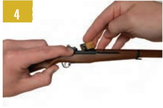
Pull back on bolt to reveal clip loading area. Insert clip with dummy rounds facing the barrel. Push down until the bolt is clear and able to slide.
