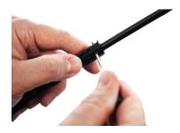
Screw barrel (C) and receiver (A) together with medium screw into hole below front sight.
