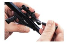
Place scope onto receiver, tighten with screwdriver.
