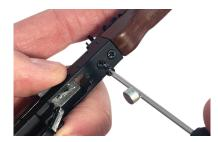
Screw the two medium-length screws into bottom of receiver to secure barrel in place.
