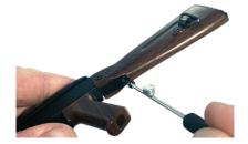
Attach the stock (J) and tighten top and bottom witht the two large screws.
