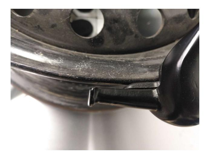
It is important that the rear of the head sticks out slightly past the rim edge and not inline with the rim.
