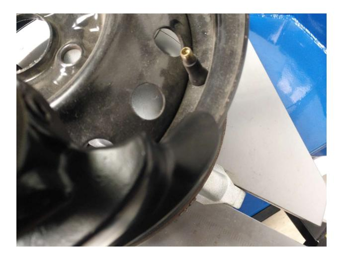
After proper head alignment is achieved make sure all 4 Allen keys are tight to prevent head twist and then unlock head and tighten the main bottom bolt.
