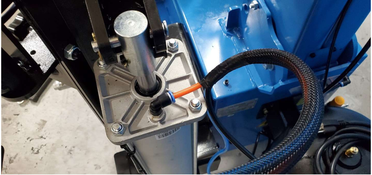
The orange tube connects to the top of the assist arm cylinder and the blue tube to the bottom.
