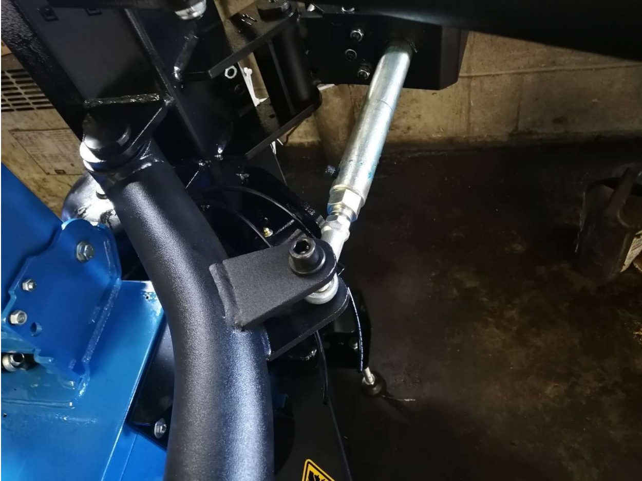
Attach the arm lock to the arm as shown.
