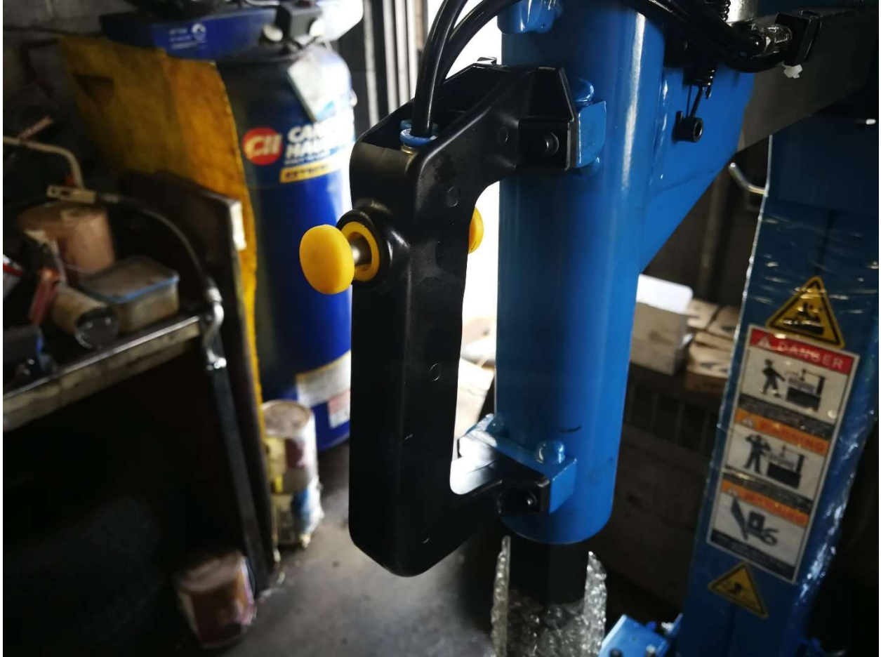
Attach the handle with screws provided in tower arm.
