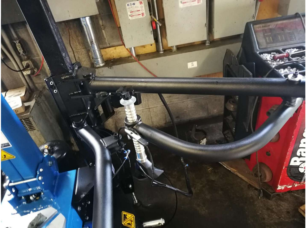
Assemble the following bead assist arm as shown. Please add grease to all joints before assembly. Pin is in the assist arm.
