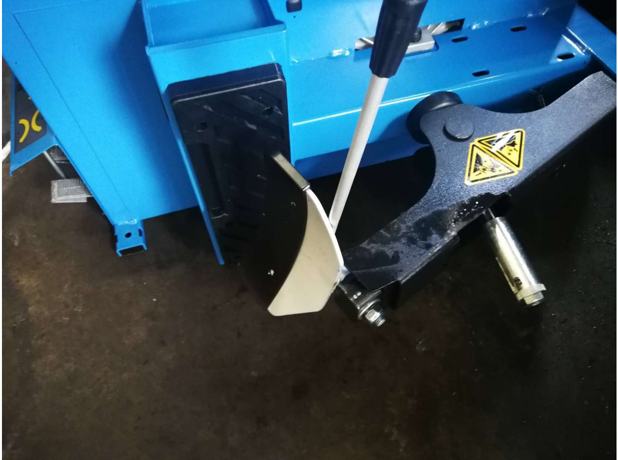
Straighten blade and tighten nut just until blade will hold position.
