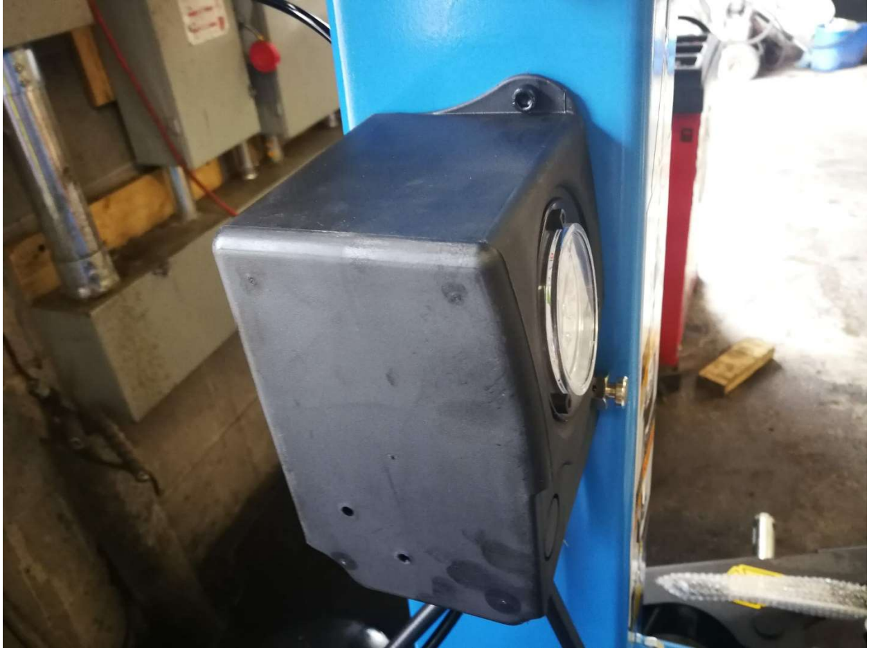
Attach the tire inflation box with screws provided in the tower.
