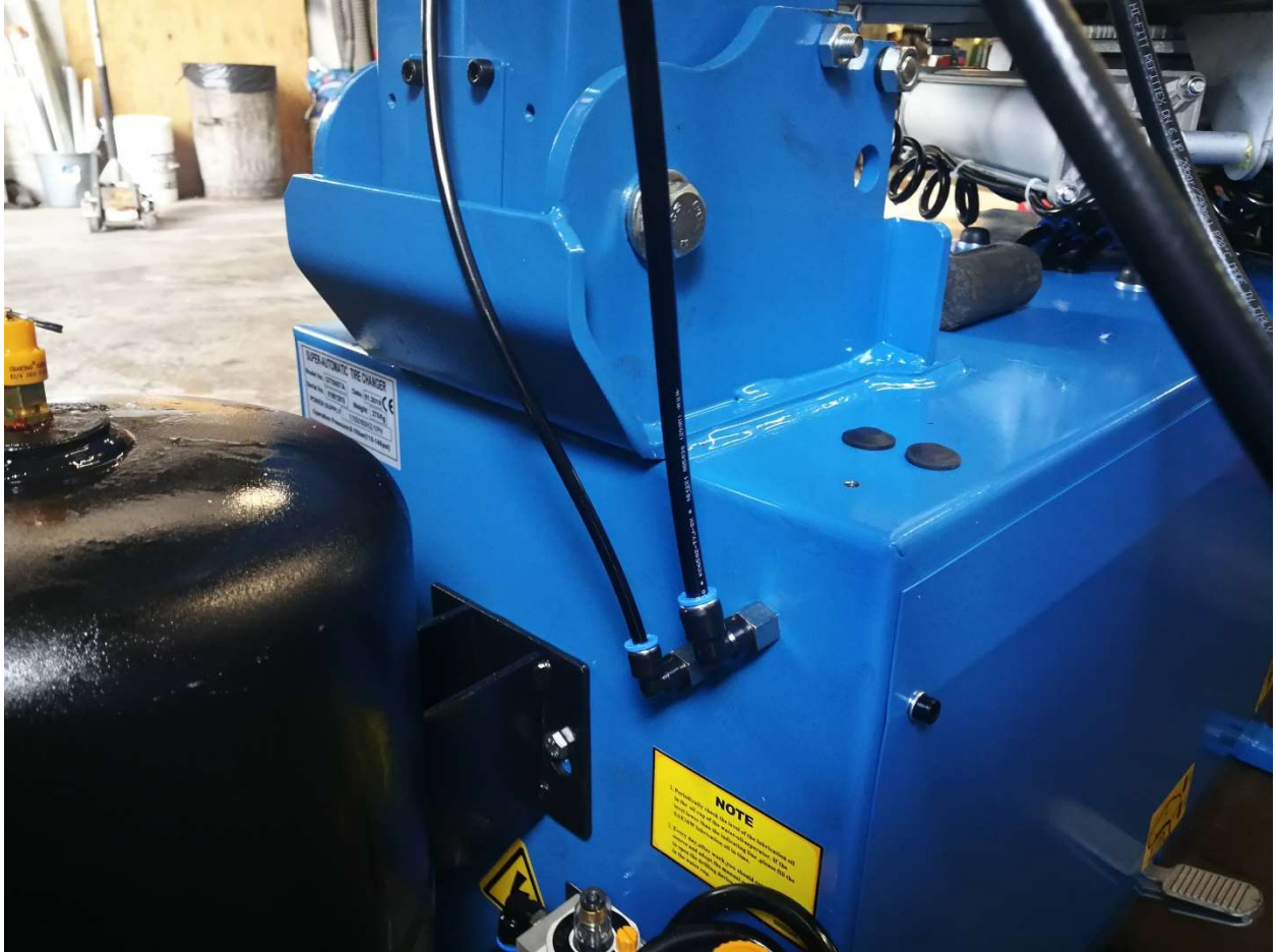
Attach the supply line to the second fitting.
