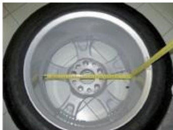
Figure F3.3.1 Example of manual measuring of the external diameter (da2) of the wheel in the ALS1/ALS2 Programme Type
