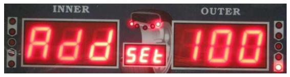
Use your hand to rotate the tire until all 5 of the lights in the **OUTSIDE UNBALANCE POINT** are on, as shown here:
