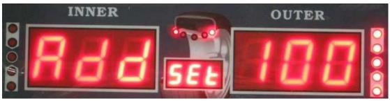
Then place the 100gram or 3.5 Ounce weight that came with the machine at 12 0'clock on the outside of the rim using the provided wheel hammer. 100 grams = 3.5 ounces so either weight is ok. Remember that at anytime you can switch from Grams to Ounces and back by just pushing the **C** button.
