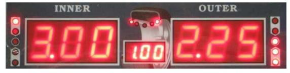
Use your hand to rotate the tire until all 5 of the lights in the **OUTSIDE UNBALANCE POINT** are on, as shown here:
