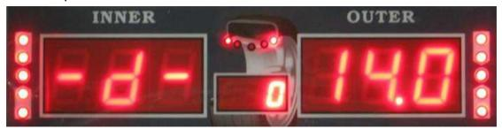
This parameter measures the rim size. This is the D parameter. Use the plastic caliper provided with the machine to measure the width of the rim. Touch the caliper to the edge of the rim on one side to measure the rim size. Use the **UP** or **DOWN** key to enter the parameter. Do not multiply this number like you did with parameter A. Simply enter the number as shown on the caliper.
