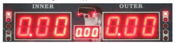
You zeroed out both sides and successfully balanced the wheel.
