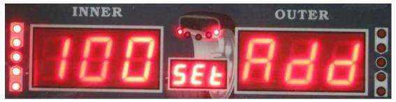
Then place the 100gram or 3.5 Ounce weight that came with the machine at 12 0'clock on the inside of the rim using the provided wheel hammer. 100 grams = 3.5 ounces so either weight is ok. Remember that at anytime you can switch from Grams to Ounces and back by just pushing the  $\bf C$  button.
