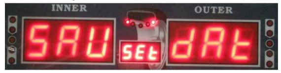
After showing this screen, the machine will automatically return to the initial balancing screen. You have successfully calibrated the machine and the data was saved automatically.
