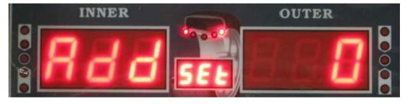
Now close the plastic hood and spin the wheel. If you have the guard control setting to "On" then the wheel will spin when the hood is closed. If you have the guard control setting is set to "Off" then you must push the **START** button to spin the wheel.
