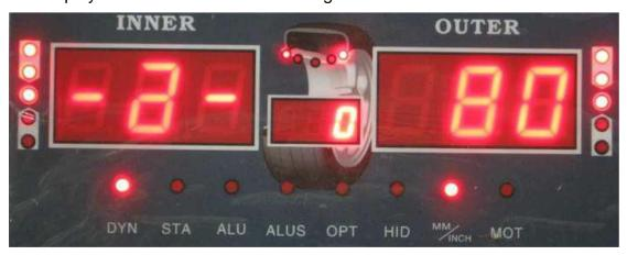
The number in the **OUTSIDE UNBALANCE DISPLAY WINDOW** may be different if you have used the machine before.
