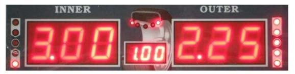
Then place the 2.25 Ounce weight that came with the machine at 12 0'clock on the outside of the rim using the provided wheel hammer. After placing the weight, close the hood and spin the wheel. The following screen will appear:
