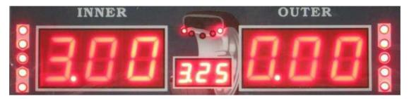
Now place the 3.00 Ounce weight that came with the machine at 12 0'clock on the outside of the rim using the provided wheel hammer. After placing the weight, close the hood and spin the wheel. The following screen will appear:
