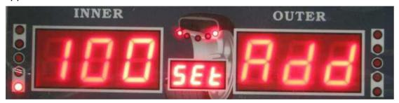
Remove the weight from the outside of the rim. Use your hand to rotate the tire until all 5 of the lights in the **INSIDE UNBALANCE POINT** are on, as shown here:
