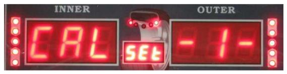
Now push and hold the **ENTER** button. While pushing and holding the **ENTER** button, push and hold the **FINE** button. The following screen will appear:
