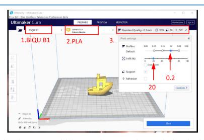
Select the printer model that users has previously set and select the slice parameters.
