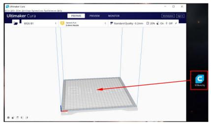
Drag the model file of stl format into the slicing software window.
