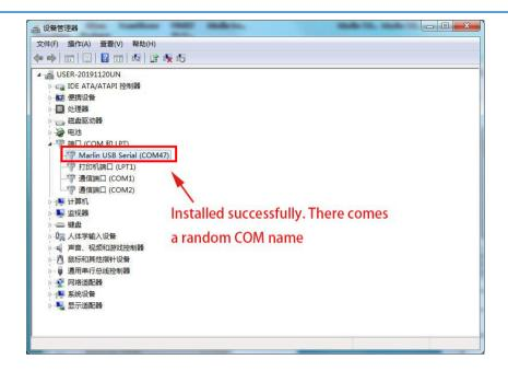
After successfully installation, you can see a random port named "Marlin USB Serial (com47)". 47 is a random number. Different numbers may appear according to different PC types. (If it is the same computer and the same printer, the port number will remain unchanged.) This port will be used for data communication between the printer and the computer.
