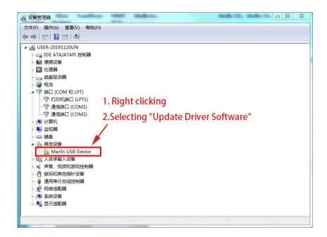
Turn on the power of the 3D printer, and connect the computer to the 3D printer through the data cable. Right-click "This Computer" → "Properties" → "Device Manager", and then the window will show above. If there is a yellow exclamation mark or question mark shown in the box, users need to manually install the driver. If not, it means that the driver has been installed automatically, no need to perform the following driver installation steps.
