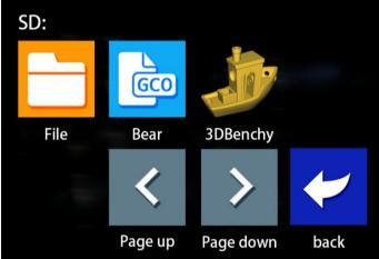
Choose from the touch screen homepage ① "Print"  $\rightarrow$  ② "TFT SD", and when selecting the slice file saved in the TF card, users will see the interface of the print file has been changed. The outputted sliced files will display thumbnail icons, while without outputted sliced files will not display thumbnail icons. Users could select the slice file they want to print at a glance.
