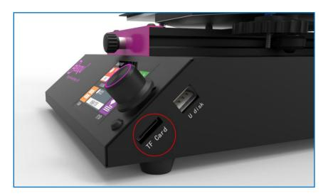
Put the G-code file from TF card in the card slot. (As shown in the figure)
