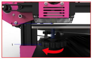
In the same way, touch the "second point", "third point" and "fourth point" on the screen in turn, and use the same method to turn the hand-screw nut under the platform to manually level the platform.
