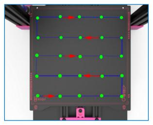
After finishing the automatic leveling, user can click "Repeat" in the previous operation interface, the printer starts printing, and the users can evaluate the leveling effect of the platform based on the printing effect to optimize the next step.
