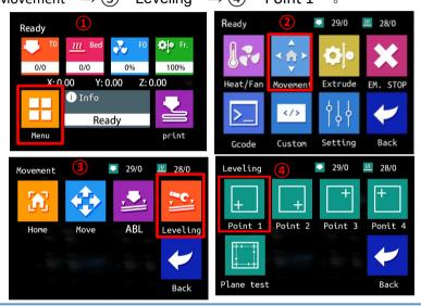
**Step 2** When the nozzle moves to the "first point" position(as shown below ), and user put a piece of A4 paper under the nozzle. Twisting the hand screw nut to make the nozzle just contact with the A4 paper and that the A4 paper can move smoothly with slight friction.
