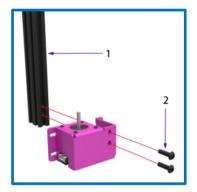
There is a M4 threaded holes on another 2040 aluminum profile. When installation, users make the threaded hole face the metal sheet part.
