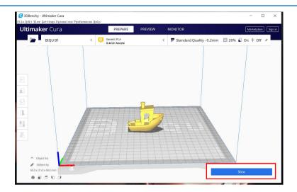
The slicing software starts slicing the model.
