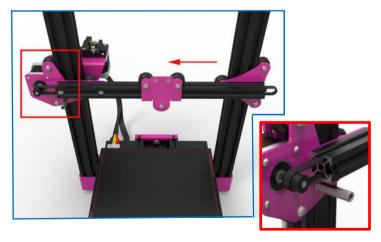
Installing the belt onto the 2020 aluminum profile.
