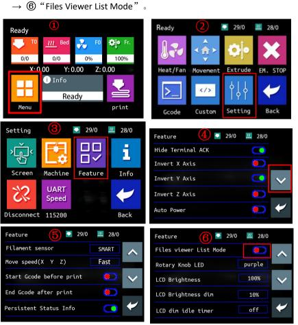
When "Files Viewer List Mode" option turns red, it means that the machine has opened the file browsing mode.
