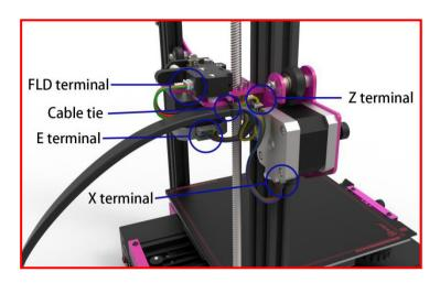
As shown above, installing the 4 in 1 terminal wire to its corresponding position. Then there are two key slots on the metal sheet part. Users can use a cable tie to fix the terminal wire through them.
