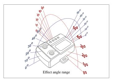
For best results, the sensor base should be flat relative to the floor or the roof of the car. Location should be central and rigid within the vehicle.
