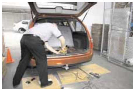
9. Drill access hole in a high point to avoid road debris in rear of car. Apply zinc based anti-rust paint. Insert rubber grommet to avoid chafing cables.
