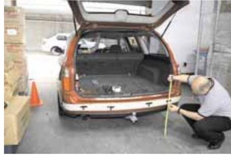
6. Mark the heights of all the sensors. The VX Commodore bumper is least curved at 510mm from the floor.
