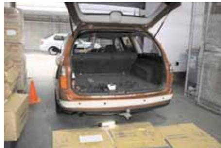
8. When all holes are drilled, remove masking tape and insert heads into each hole. Secure all cables inside bumper.
