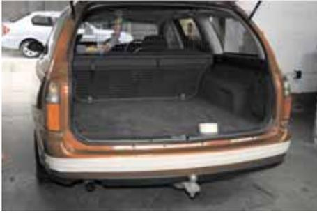
1. Mask rear bumper both below and above approximate sensor locations. This will help with marking and reduce scratching the bumper.
