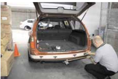
5. When satisfied with results, measure and separate heads with greater accuracy. This car has a 300,600,300 split between the heads (aligned central to tow bar).
