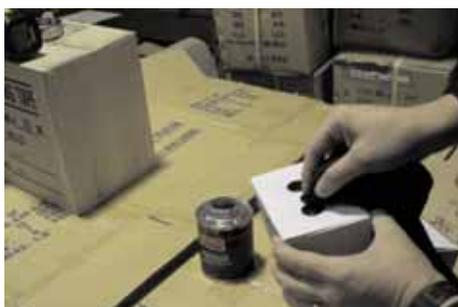
5. Use PREPWASH to remove any grease, oil & dust. Ensure the clean surface is not touched again until after the painting procedure is complete. Solvent fluid must be enamel compatible.
