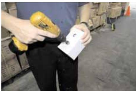
1. To mash the sensor heads, drill two holes in cardboard box that the sensors are supplied in. Use the hole saw supplied.
