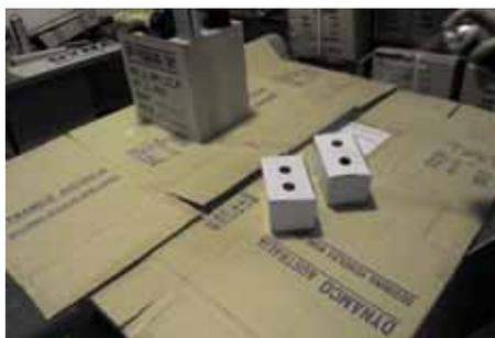
6. Apply FLEXI-PRIME plastic adhesion promoter. Two light coats are preferred to one thick coat \*\*\*. Leave in dust free location to dry.
