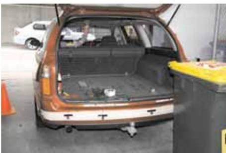
4. Temporarily wire up all connections and test coverage by moving firm object in and out of the field. Sensors should respond only when object is within the car profile.
