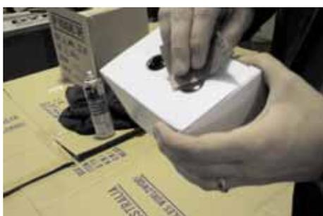
4. Use a very (very) fine grade of wet and dry abrasive paper to remove the shine of the heads.
