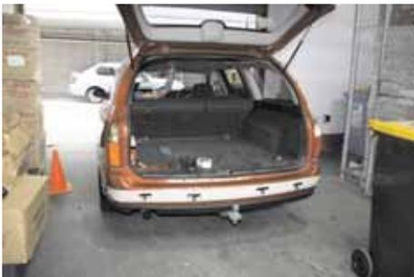
3. Temporarily mount each sensor head in it's approximate position using tape. Notice the centre heads have been spread further to allow the ultrasonic field to miss the tow bar.
