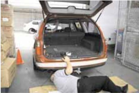
2. Check behind bumper to ensure sensor heads will have enough clearance and cables can be fixed to anchor points.
