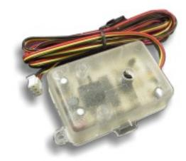
Cable tie or screw the sensor against rigid structure within vehicle. The rigid structure must pass any all vibration to the sensor, the steering column is an excellent example.
