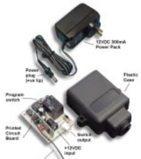
The kit is not supplied with any remote controls. The client's alarm or immobiliser remotes must be programmed into the garage door controllers memory. The controller carries sufficient memory to track five "Code Hopping" remote.
