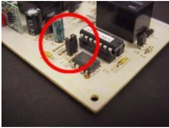
JUMPER CLOSED (REPLACED)
