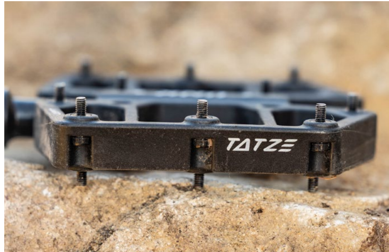
The LINK Composites offer a lot of grip, but also poor self-cleaning.
