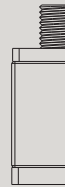
U5 (ADR7538) Fit 1-3/8 Square Tube Exp. 1.360 - 1.425 1/4 Square Metal Top Square Rubber 1/4 Metal Base
