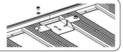
( D ) Insert the end of the Additional Slat which does not have the Plastic End Cap form Step 2A into the "U-channel" of the Side Profile directly opposite the Joint. The Slat must be inserted with the Nyloc Nut facing upwards. The other end of the Slat with the Plastic End Cap can be rested on the Inter-slat Bracket.
