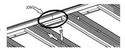
Place the Inter-slat Bracket (Item 1) over the two Hex Bolts inserted and loosely fasten to the rack using two M8 Flat Washers and two M8 Nyloc Nuts (Items 4 &6). The Inter-slat Bracket must still be able to slide.
