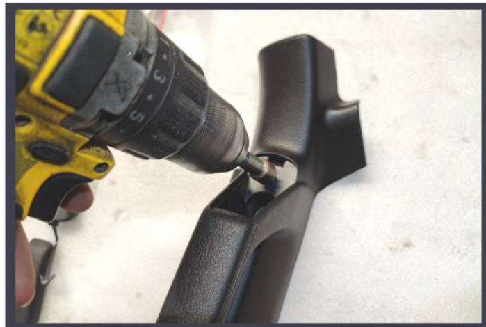
Drill a 20mm hole in the handle for the cable of the switch panel.
