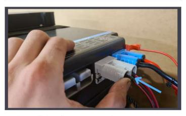
Step 1: find the charger's cable that goes to the battery and cut off the plugs or eye ends.
