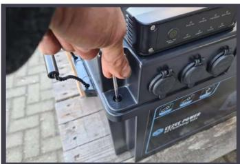
Use the supplied Allen bolts to attach the lid to the box. You have now successfully installed the battery, hooray!
