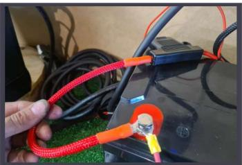
Connect the black cable to the negative pole of the car battery. Attention: never disconnect the original negative pole from the car battery as this can completely reset the car's computer.
