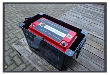
Stick 2 pieces of double-sided tape to the bottom of the box to keep the battery from sliding around inside the box. Then put the battery in the box.
