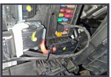
Place the Add-a-Fuse tool in the original position of the car's fuse.
