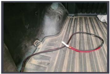
Find the most convenient way to run the cable from the Battery Box to the car battery. Make sure to put the cable end with the fuse holder near the car battery and the cable end with the painter's tape near the Battery Box. Keep the cable away from the exhaust system and beware of turning parts. Use enough cable ties to firmly hold the charging cable in place.
