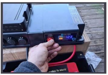
Test the battery functionality by turning on the main switch and the battery monitor. If the display doesn't show a voltage you need to check and correct your connections.
