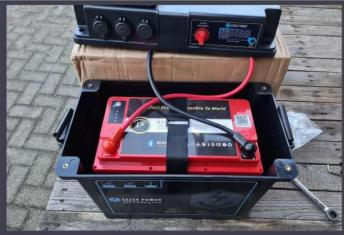
Connect the red cable to the positive terminal of the battery and attach the rubber cap. Connect the black cable to the negative terminal of the battery and attach the rubber cap.
