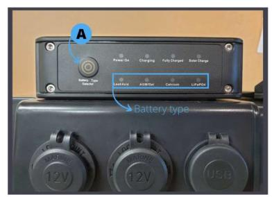
Step 1: check if the battery is in safety mode by short pressing button A. If every short press changes the battery type, the battery is in safety mode.
