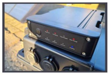
The built-in charger has a few indication leds to check the charging status.
