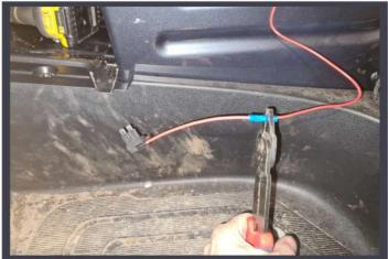
Place the car's fuse in the bottom place of the Add-a-fuse tool. Crimp the Add-a-Fuse tool onto the ignition cable.
