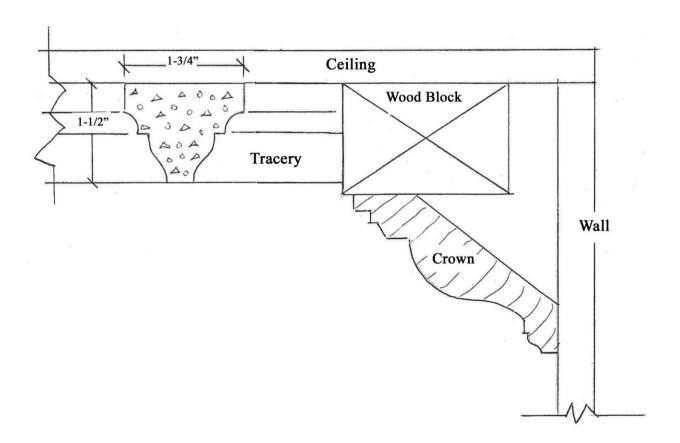
This sketch illustrates how a wooden block can be placed on the ceiling to serve as a soffit to receive the tracery units as well as the upper part of the crown moulding. The result will be a very finished look. We recommend a block that's 1-5/8" x 1-5/8" for these tracery patterns. For our Old English and Italian coffered ceiling panels, a block of the appropriate depth would be used as a soffit. Of course, this works only in rooms that don't have crown mouldings already in them.
