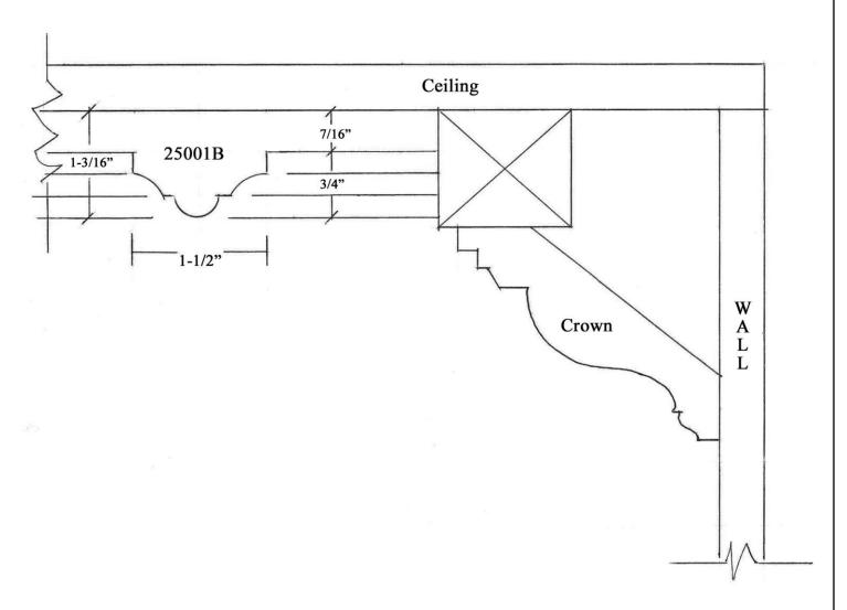
This sketch illustrates a solution for terminating our 25001B and 25001C ceiling panels up against the walls of a room using the block & crown method. Of course, this works only in rooms that don't have crown mouldings already in them.
