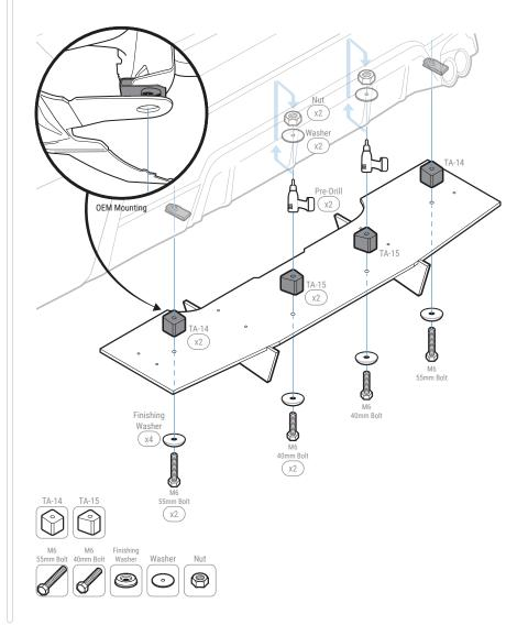
Remove the OEM Push Pins under the bumper located on the Driver and Passenger Side
