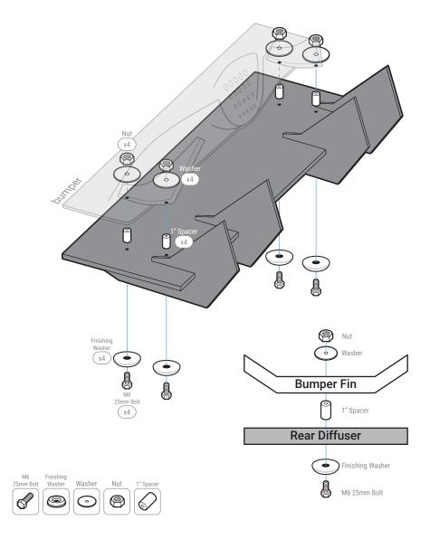
Drill through the center of the Rear Diffuser into the bumper
