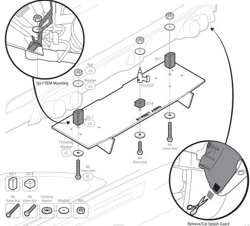
Remove the Push Pins located under the bumper near the rear wheels (see diagram below) NOTE: We recommend removing the Splash Guard to get access behind the bumper
