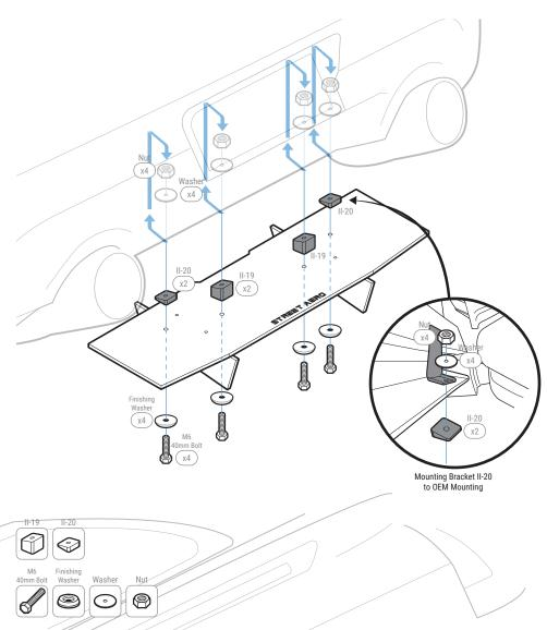
Remove the OEM Washer Bolt located under the bumper near the rear wheels
