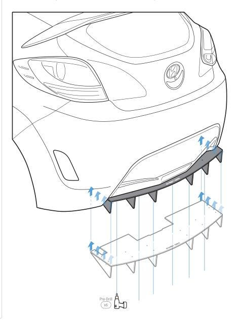
Secure the Rear Diffuser to the bumper with M6 25mm Bolt, Finishing Washer, Washer, and Nut
