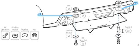
Attach and secure Mounting Bracket FD-44 and FD-45 to the Side Panel with M6 16mm Bolt, Finishing Washer, and Nut
